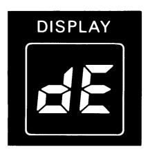
This flashing code tells you something's wrong with the defrost system—keep doors closed to retain cold and call for service. Code flashes until problem is corrected.
